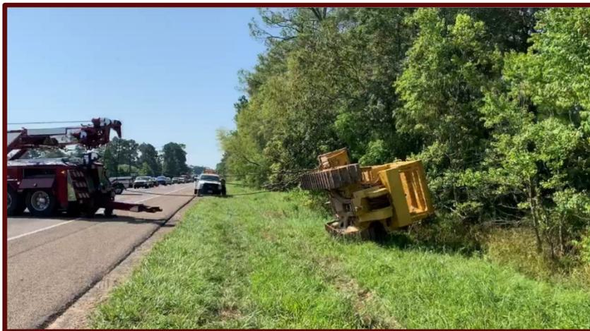
**Figure 2:** Wrecker with winch attached to dozer, pulling it over onto its tracks.
